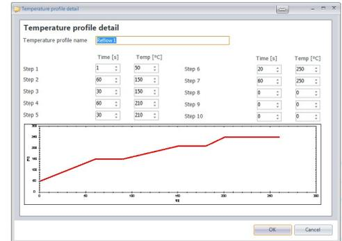
Temperature Profile for Paste Test
